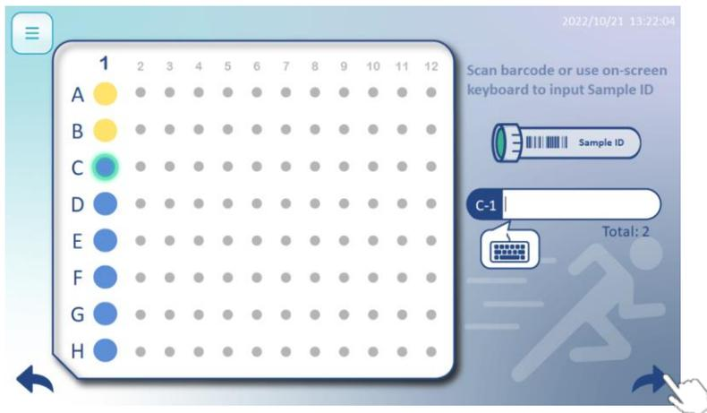
A circle turns yellow when inputs sample ID successfully. Then it moves to next sample ID automatically. E.g. A1→B1, B1→C1 etc. Press arrow to proceed next page.
