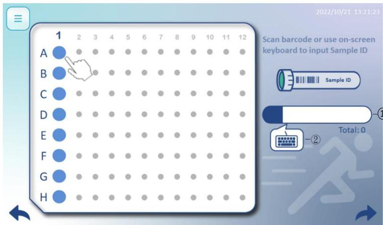
Press a circle(A1~H1) to input sample ID by using 1-D barcode ①barcode or ②manual type in.
