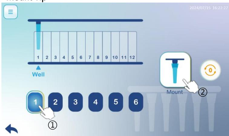
Please apply with spin tip assemble box onto the heating plate inside the SW8. ① Select desire lane and ② press on “Mount” to pick up spin tips.
