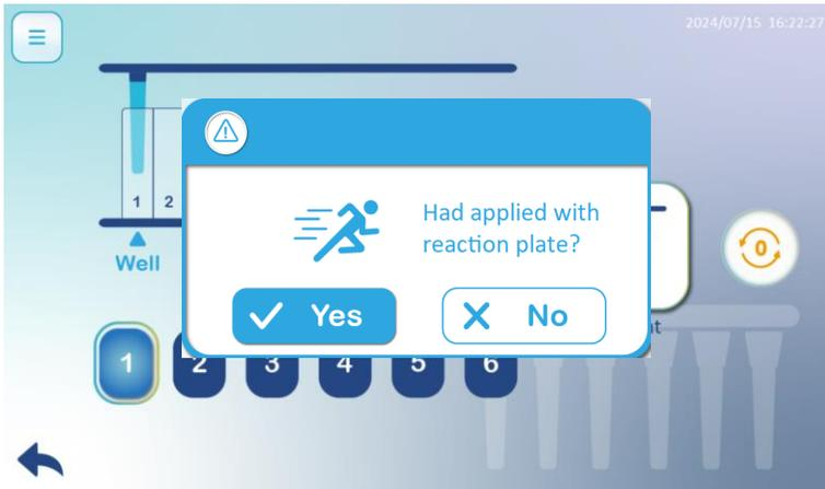
After picking up the spin tips, make sure to replace the spin tip assemble box with prepared reaction plate. Click on "Yes" to proceed or "No" if the plate is not ready.
