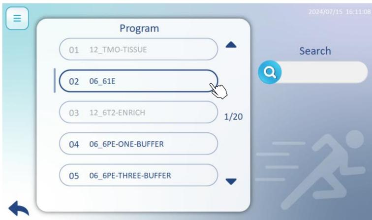
Switch 8 has an impressively large store of 100 programs. Choose program that in line with your reagent kit. Type in key words in search box to look for programs if needed. Number indicated with "06\_" or "12\_" refer to different types of program with 06 step program or 12 step program.
