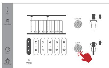
Tap "Tip" → "Eject" to eject the tips if choosing Auto Tube. Withdraw the finished plate.
